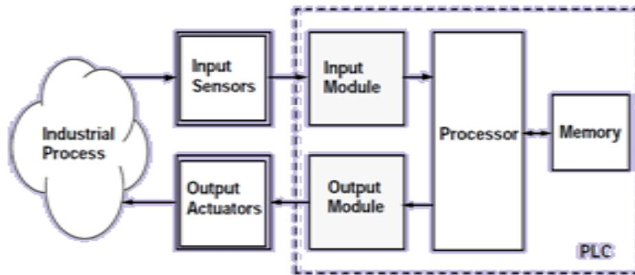
Figure 2 PLC Block diagram
