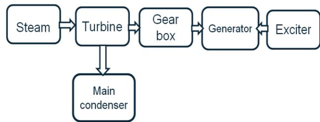
Figure. 1 Block diagram of Turbo Generator
