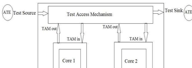
Fig 1:- Modular Structure of a SOC.
