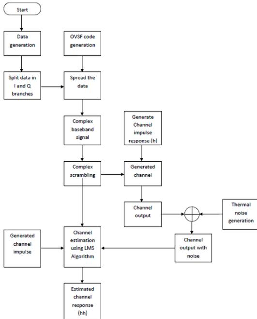
Fig. 3 Flow chart for Channel Estimation
