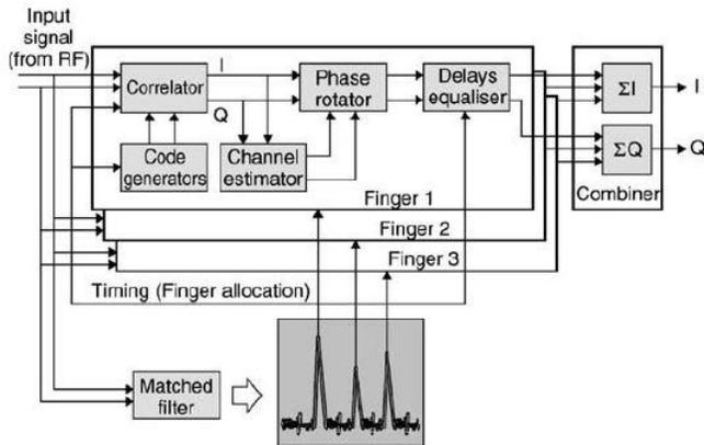
Fig. 1 Block diagram of the CDMA Rake receiver
