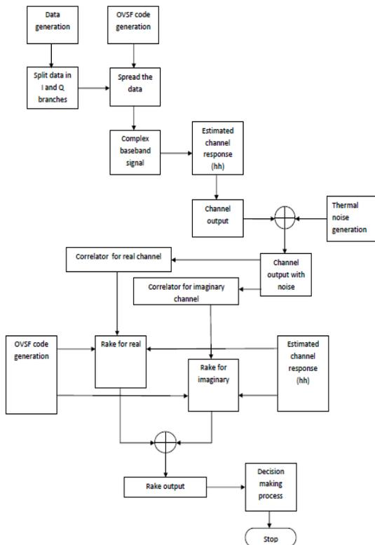
Fig. 4 Flow chart for Rake Receiver
