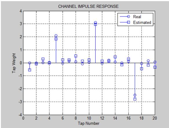
Figure 5 channel impulse response (no of multipath=3)
