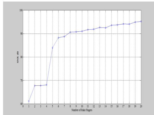
Fig. 9 SNR (dB) for different number of Rake Fingers
