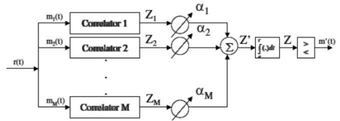
Fig. 2 An M-branch Rake receiver
