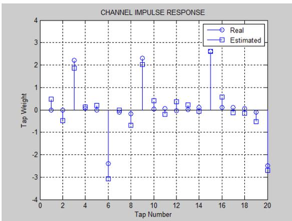
Figure 6 channel impulse response (no of multipath=5)
