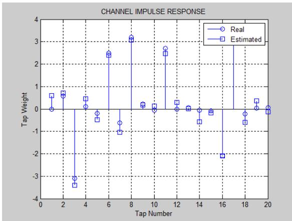
Figure 7 channel impulse response (no of multipath=9)
