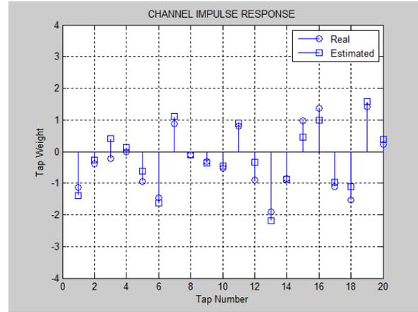
Figure 8 channel impulse response (no of multipath=20)
