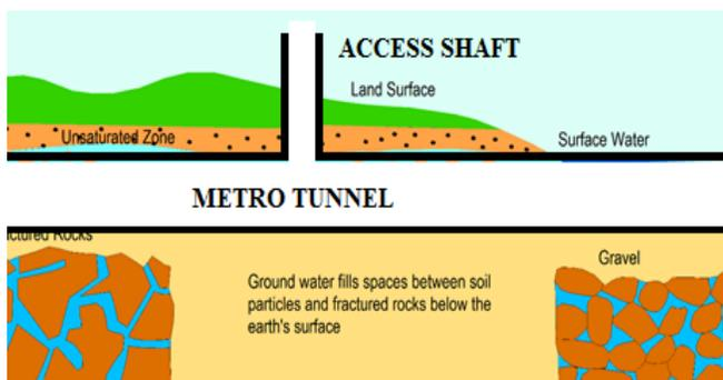
Figure 1b: Underground tunnel causing disturbance to aquifer
