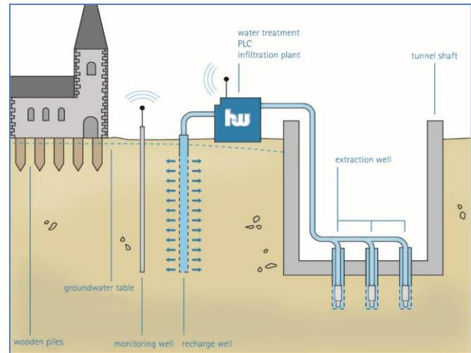
Figure 7: Schematic diagram of Hölscher's groundwater management concept.
