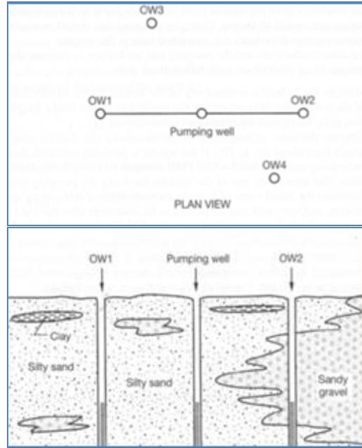
Figure 3(a&b): Number and position of observation wells in plan and elevation.
