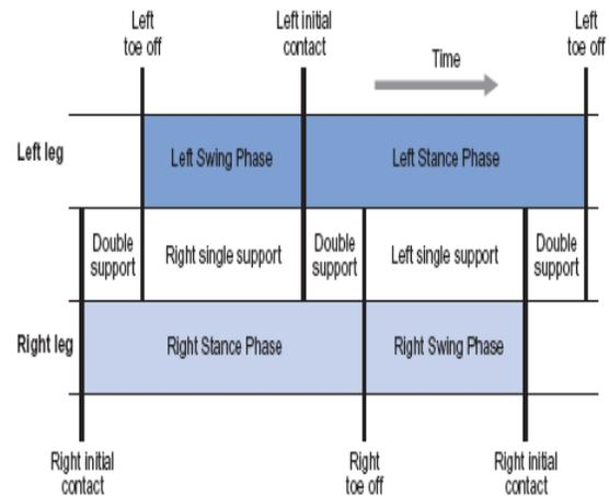
Figure 3: Sub phase Of Stance and Swing[8]
