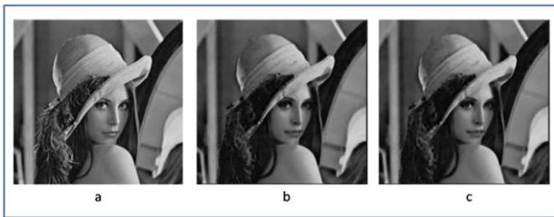
Fig. 7 Processing with Minimum filter
