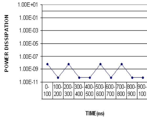
Figure 5: Power dissipation during write operation
