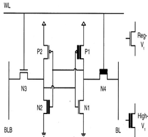
Figure 1: Asymmetric 6T SRAM cell.
