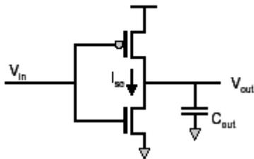
Fig. 2: Short Circuit Power Dissipation
