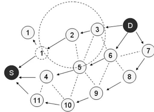
Fig -3 B-RREQ from Destination to Source Node
