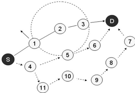
Fig 1 RREP Delivery Fail in AODV
