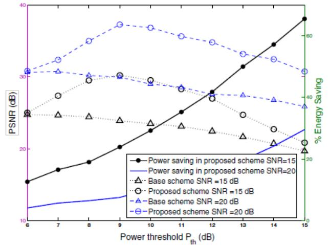
Fig 7. Energy saving PSNR with respect to threshold power  $P_{th}$
