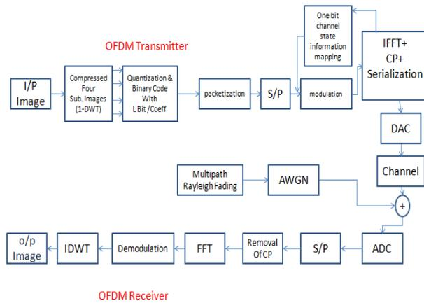
Fig 3. DWT image transmission and reception on OFDM
