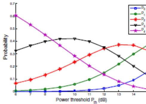
Fig 5. Probabilities associated with the lost packets in different fading channel condition
