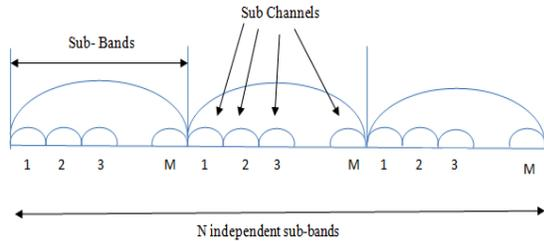
Fig 2. The sub carrier model in the block fading channel of OFDM system
