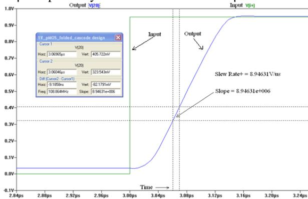
**Figure 3: Positive Slew rate of rail to rail Op-amp**
