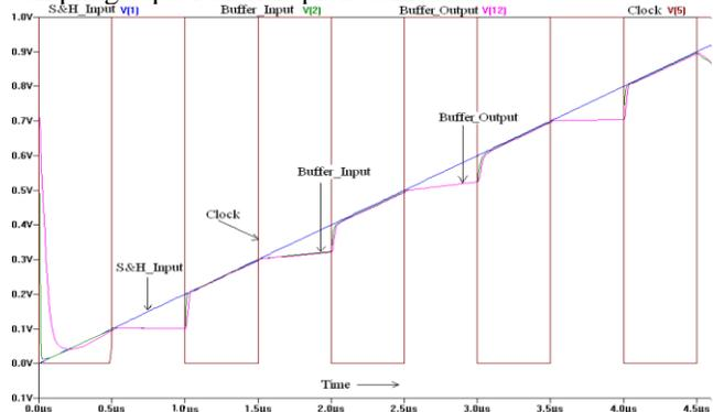
**Figure 7: Sample & Hold circuit response to a ramp input signal.**
