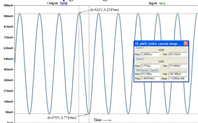
**Figure 6: Transient response of a rail to rail Op-amp connected in unity gain configuration for sinusoidal signal of 0.84 V<sub>pp</sub>**
