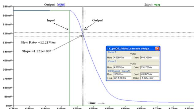
**Figure 4: Negative Slew rate of rail to rail Op-amp**
