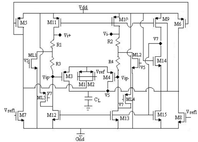
**Fig.1. Proposed Circuit for rail to rail operation**
