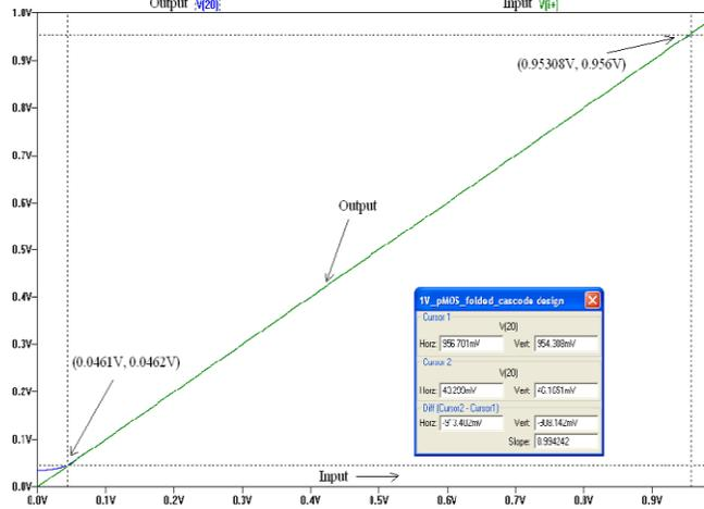
**Fig.5 Transient response of a rail to rail Op-amp connected in unity gain configuration**
