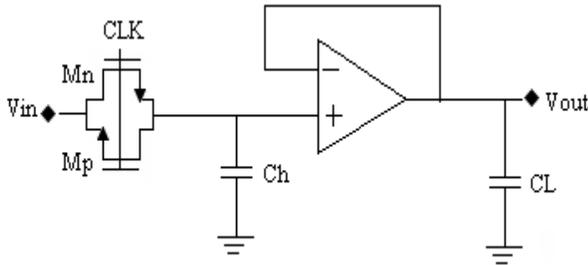
Fig.2. Open Loop Sample and Hold Circuit
