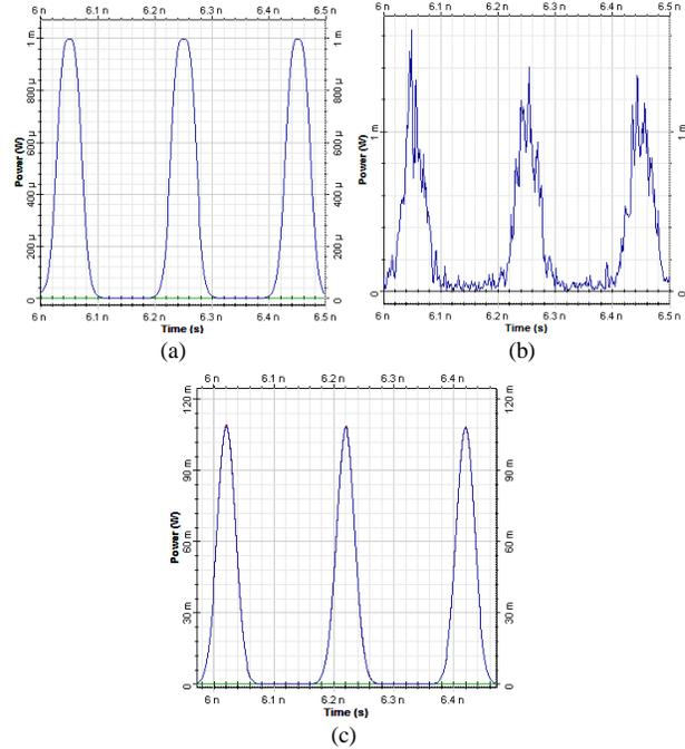
Fig.5. Waveforms for (a) Transmitted signal, (b) Degraded signal, and (c) Regenerated signal
