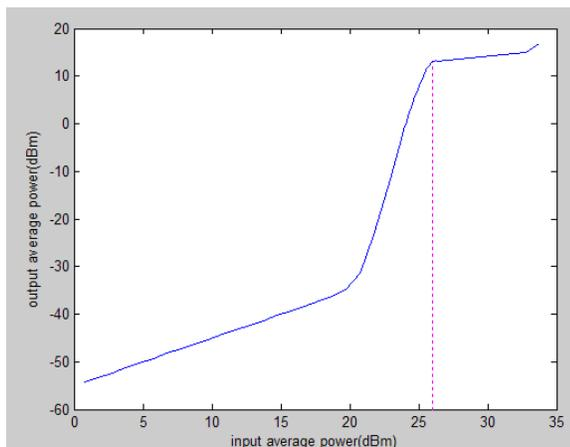
Fig.7. Power Transfer function of the 2R regenerator
