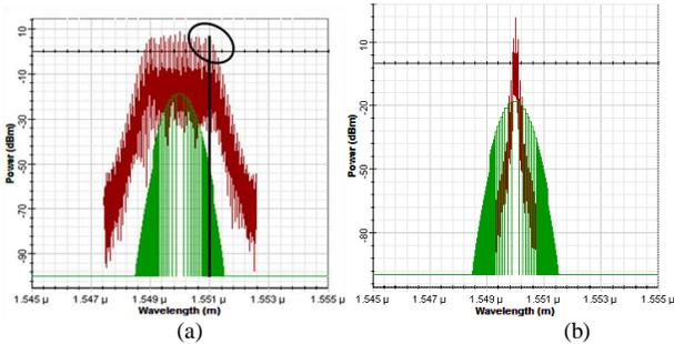
Fig.4. (a) The spectrum of the degraded signal, and (b) The broadened spectrum induced by SPM effect
