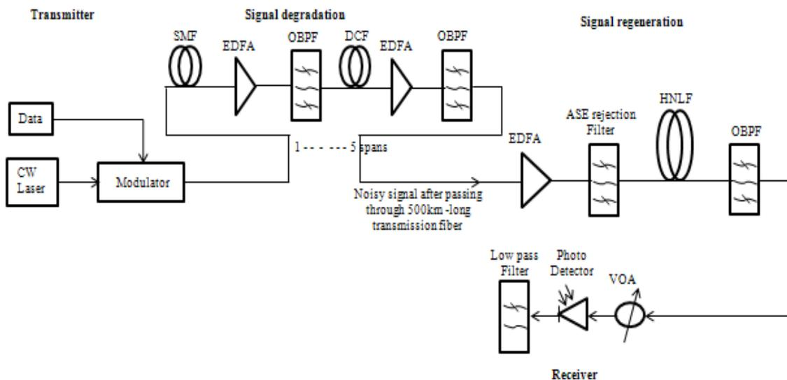
Fig.1. Block diagram of the proposed design work
