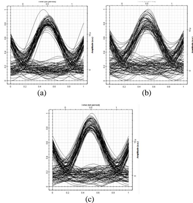
Fig.6. Eye diagrams for (a) Back to back system, (b) without regenerator after passing through 500km transmission fiber, and (c) after regeneration at approximately 10<sup>-9</sup> BER
