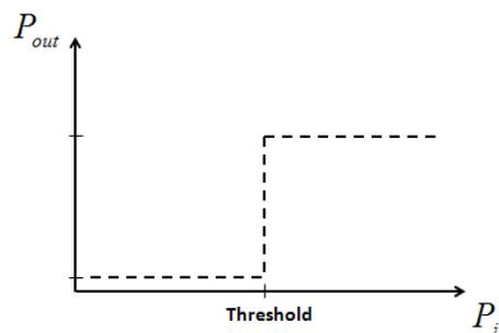
Fig.2. Illustration of an ideal step-like power transfer function
