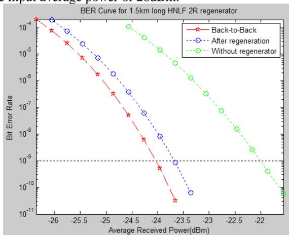
Fig.8. BER measurements for 2R regenerator
