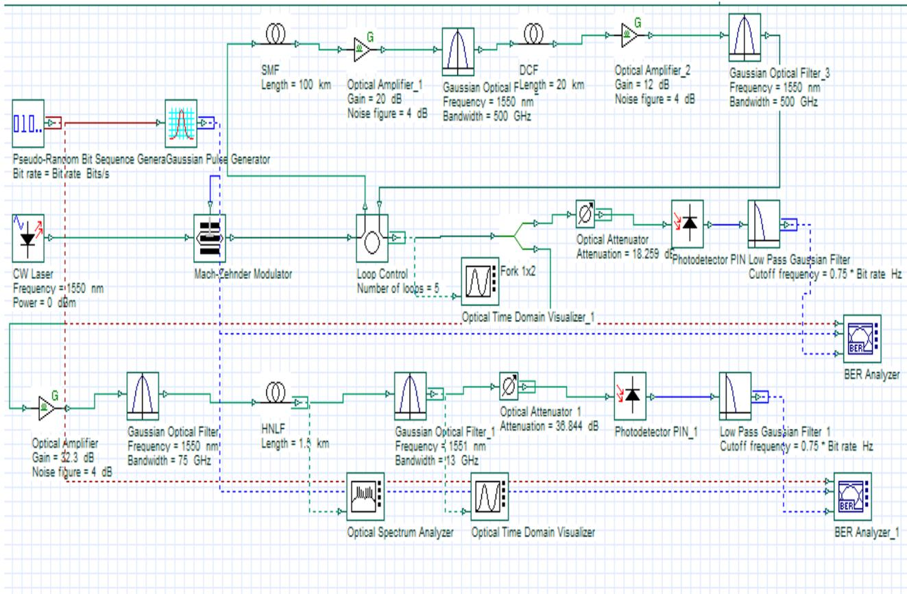
Fig.3. Simulation setup of the proposed system
