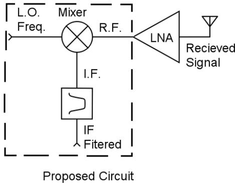
Fig. 2: Proposed combined circuit in the receiver.
