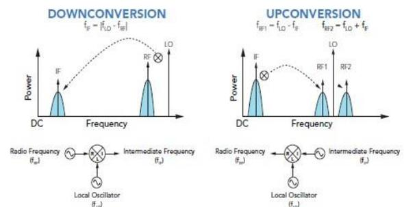
Fig. 1: Definitions of down conversion & up conversion.
