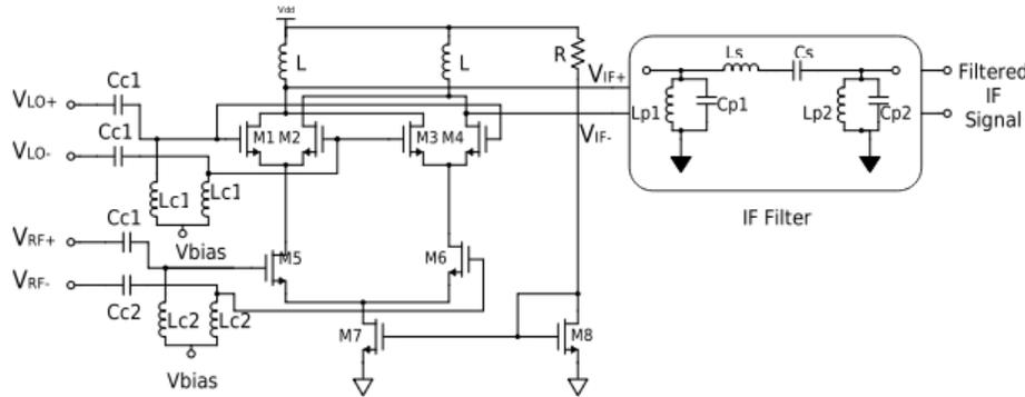
Fig. 5: Proposed combined Mixer+IF filter schematic for automotive Radar application.
