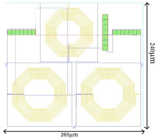
Fig. 7 RC-extracted Layout (a) CMOS Doubled balanced mixer, (b) IF filter.
