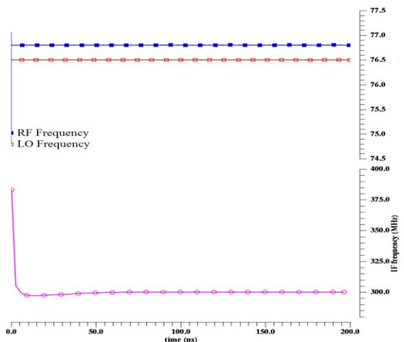
Fig. 6 Simulation analysis of Proposed circuit, (a) Voltage signal of RF, LO, and IF signal, (b) Frequency response of these three signal.
