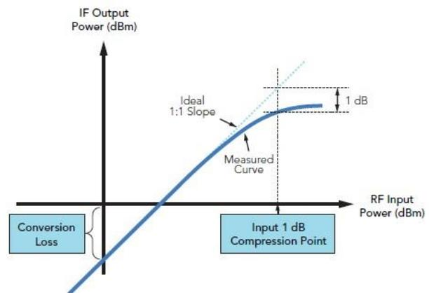
Fig. 3: Graphical representation of 1 dB compression point.
