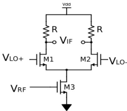
Fig. 4: Schematic of single-balanced mixer
